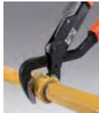
Slip joint pliers have an adjustable joint which provides a wide range of jaw openings and a firm grip on work pieces of varying shape.
