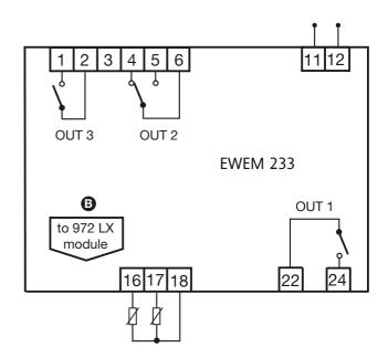
All relay outputs (OUT) from EWEM 233 module are configurable by parameter according to the following table:
