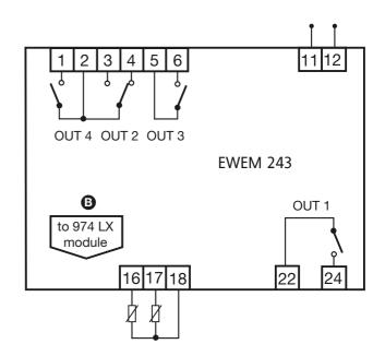
All relay outputs (OUT) from EWEM 243 module are configurable by parameter according to the following table:
