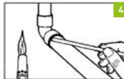
Apply heat with torch. When brazing rod melts upon contact with heated fitting, the proper temp for brazing has been reached. Remove flame & feed rod to the joint at one or two points until a ring of brazing appears at the end of the fitting.
