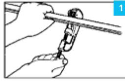
1 Cut tube to length & remove burr with file or scraper.
