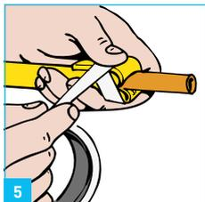
5 Secure the spliced plastic cover with tape
