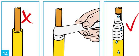
14 Exposed ends should be sealed with tape
