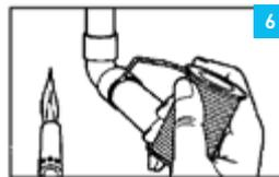
6 Apply heat with torch. When solder melts upon contact with heated fitting, the proper temp for soldering has been reached. Remove flame & feed solder to the joint at one or two points until a ring of solder appears at the end of the fitting.
