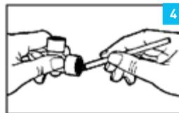
4 Apply flux thoroughly to inside of fitting.
