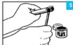
5 Apply flux thoroughly to outside of tube - assemble tube and fitting.
