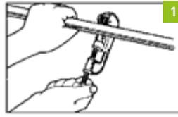
Cut tube to length & remove burr with file or scraper.
