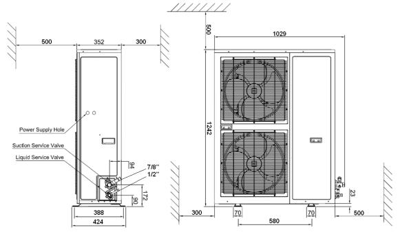
Figure 12: Fixing dimensions and distances - Dual-fan unit
