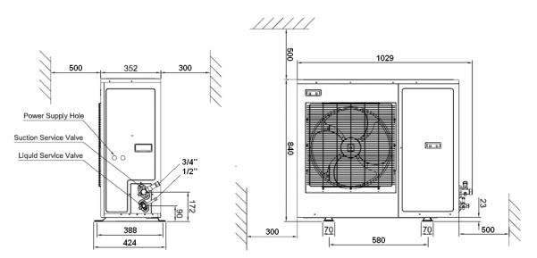
Figure 11: Fixing dimensions and distances - Single-fan unit
