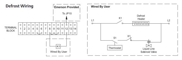
K1: Double Pole Relay/Contactor
